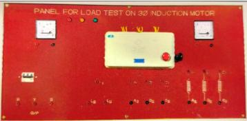
AC phase-wound slip ring Motor with pony brake loading arrangement with dial type spring balance with control panel.
